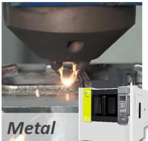
Metal powder direct energy deposition and subtractive manufacturing machine
